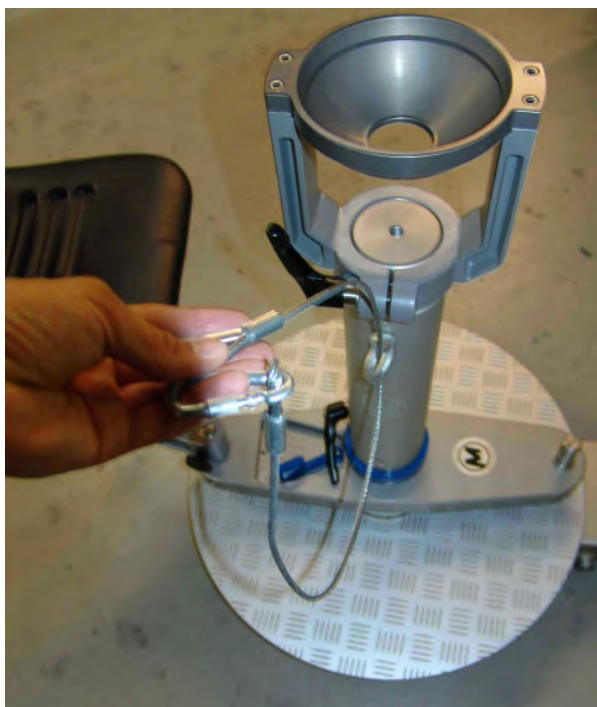
Fig. 30 Safety rope on column extension for securing loose objects
