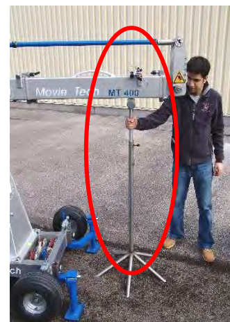
Fig. 24: Supporting the rear crane arm
