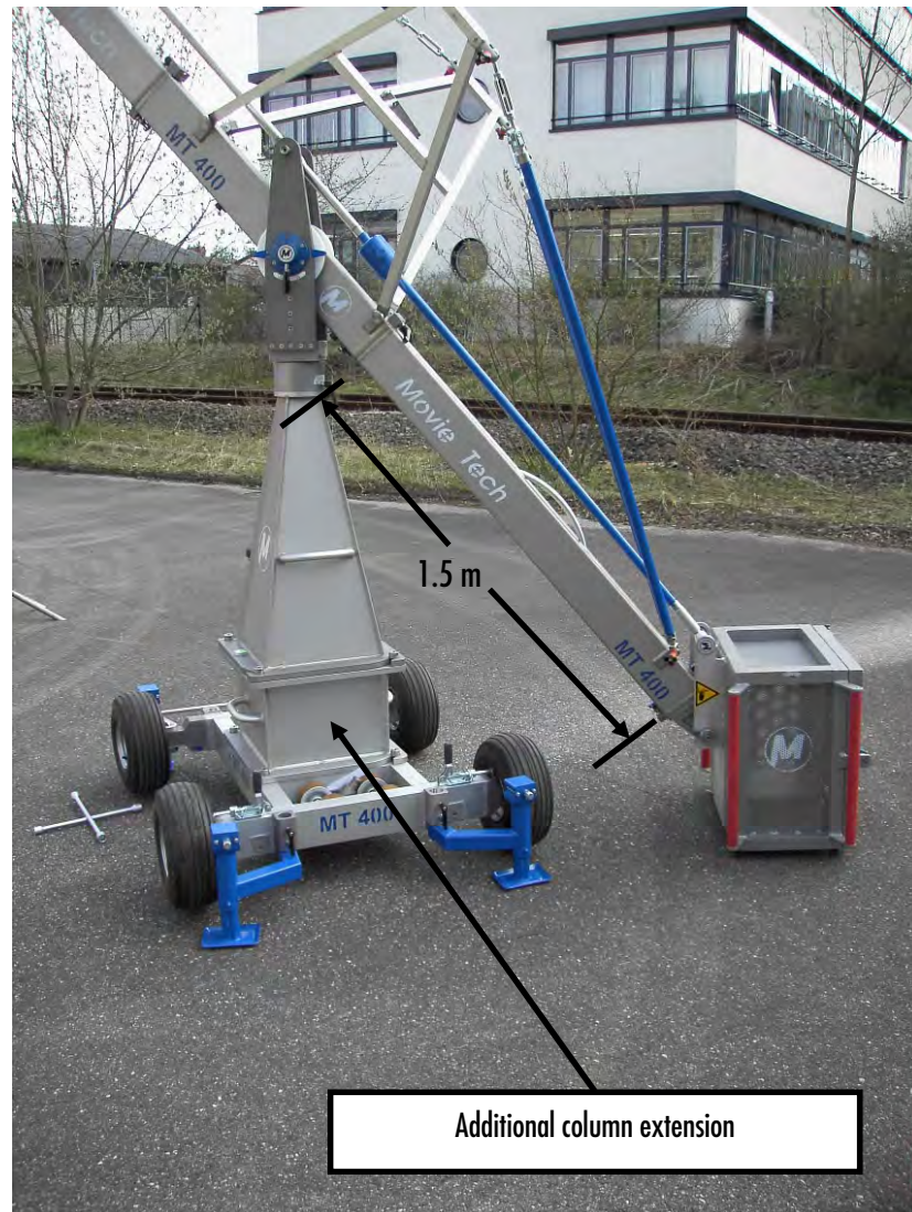
Fig. 42: 1.5 m crane element to weight basket with column extension
