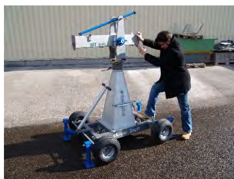
Fig. 15: Checking the crane base for stability
