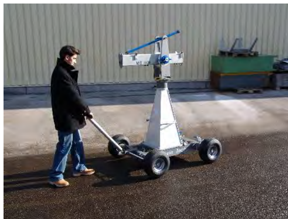
Fig. 5: Crane base with column, rotary joint and centre section
